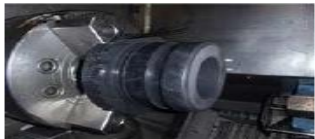
Fig.8: The outermost scrim layer being removed at Machinetek Engineering.
