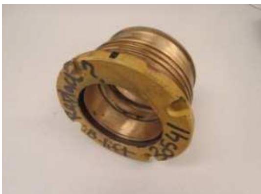
Fig. 1: The existing piston and gland that were used in the prototyping stages of the project.
